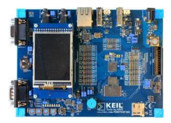
The Keil MCBSTM32F400 Evaluation Board enables you to create and test working programs based on the STMicroelectronics STM32 F4xx series of ARM Cortex<sup>™</sup>-M4 processor-based devices.
