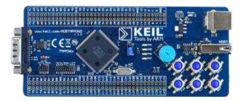
The Keil MCBTMPM360 Evaluation Boards enable you to create and test working programs based on the Toshiba TMPM360 family of ARM Cortex<sup>™</sup>-M3 processor-based devices.
