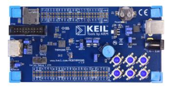
The Keil MCBTMPM395 Evaluation Boards enable you to create and test working programs based on the Toshiba TMPM395 family of ARM Cortex™-M3 processor-based devices.
