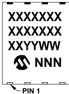
8-Lead DFN-S (6x5x0.9 mm)
