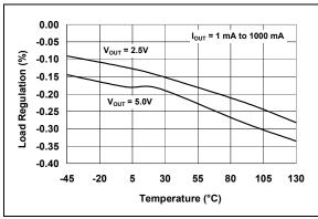
**FIGURE 2-18:** Load Regulation vs. Temperature ( $V_{OUT} \ge 2.5V$  Fixed).
