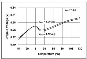
**FIGURE 2-8:** Dropout Voltage vs. Temperature (Adjustable Version).
