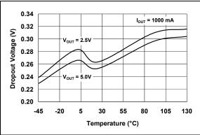
FIGURE 2-20: Dropout Voltage vs. Temperature.
