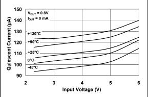
FIGURE 2-10: Quiescent Current vs. Input Voltage.
