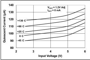
**FIGURE 2-1:** Quiescent Current vs. Input Voltage (Adjustable Version).
