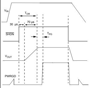
FIGURE 4-3: Power Good Timing from Shutdown.
