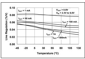
**FIGURE 2-15:** Line Regulation vs. Temperature.
