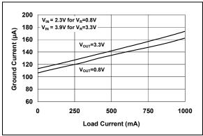
FIGURE 2-12: Ground Current vs. Load Current.
