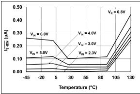
FIGURE 2-14: I<sub>SHDN</sub> vs. Temperature.
