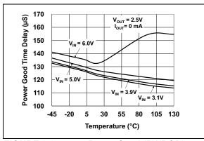
**FIGURE 2-9:** Power Good (PWRGD) Time Delay vs. Temperature.
