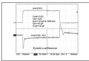
**FIGURE 2-29:** Dynamic Load Response (10 mA to 1000 mA).
