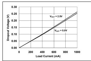
FIGURE 2-19: Dropout Voltage vs. Load Current.
