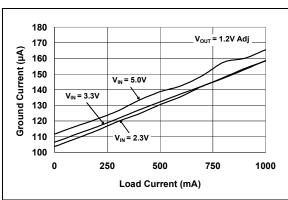
FIGURE 2-2: Ground Current vs. Load Current (Adjustable Version).
