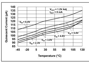
**FIGURE 2-3:** Quiescent Current vs. Junction Temperature (Adjustable Version).
