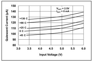
**FIGURE 2-11:** Quiescent Current vs. Input Voltage.
