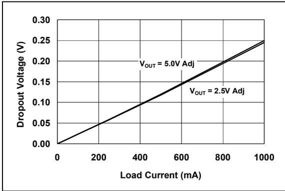
**FIGURE 2-7:** Dropout Voltage vs. Load Current (Adjustable Version).
