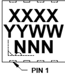
8-Lead DFN (3x3 mm)
