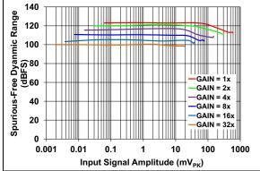
FIGURE 2-26: SFDR vs. Input Signal Amplitude.
