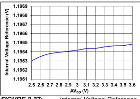
FIGURE 2-37: Internal Voltage Reference vs. Supply Voltage.
