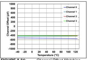
**FIGURE 2-34:** Channel Offset Matching vs. Temperature.
