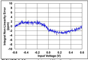
FIGURE 2-38: Integral Nonlinearity (Dithering Maximum).
