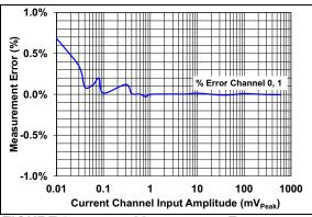
FIGURE 2-5: Measurement Error with 1-Point Calibration.
