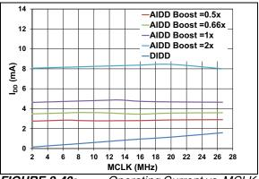
**FIGURE 2-40:** Operating Current vs. MCLK Frequency vs. Boost, V<sub>DD</sub> = 3V.
