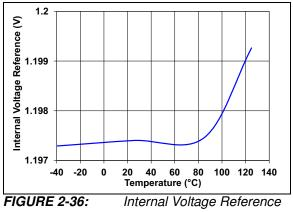
**FIGURE 2-36:** Internal Voltage Reference vs. Temperature.
