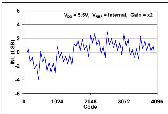
**FIGURE 2-2:** INL vs. Code ( $T_A = +25^{\circ}\text{C}$ ).
