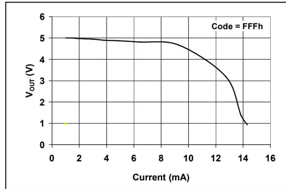
**FIGURE 2-51:** Source Current Capability ( $V_{REF} = V_{DD}$ , Code = FFFh).
