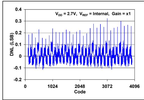
FIGURE 2-10: DNL vs. Code ( $T_A = +25^\circ\text{C}$ ).
