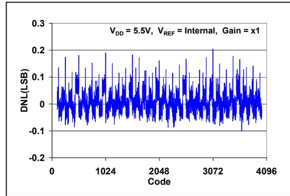
**FIGURE 2-4:** DNL vs. Code ( $T_A = +25^{\circ}\text{C}$ ).
