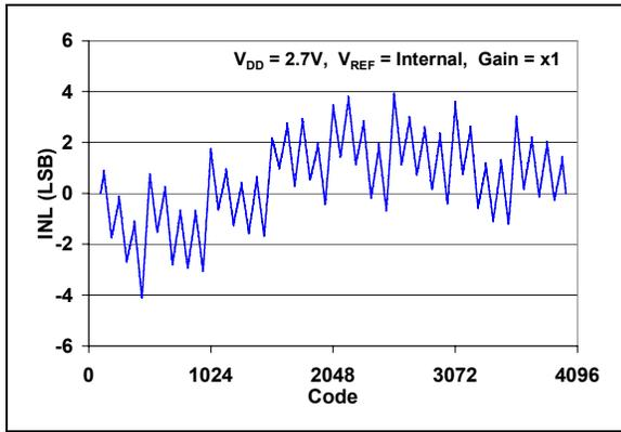
FIGURE 2-7: INL vs. Code ( $T_A = +25^\circ\text{C}$ ).
