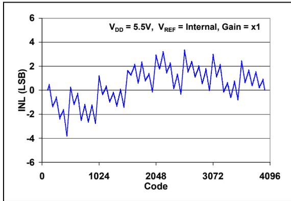
**FIGURE 2-1:** INL vs. Code ( $T_A = +25^{\circ}\text{C}$ ).
