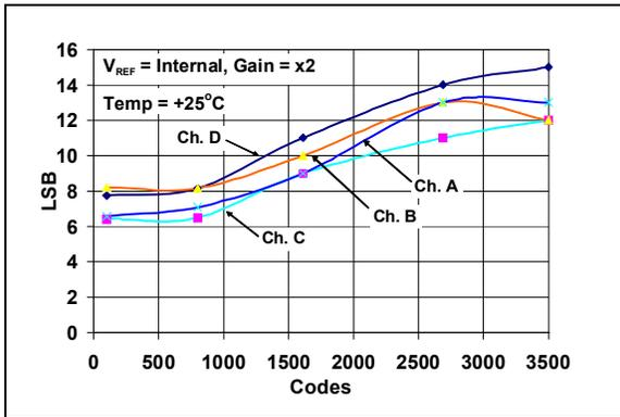
**FIGURE 2-25:** Absolute DAC Output Error ( $V_{DD} = 5.5\text{V}$ ).
