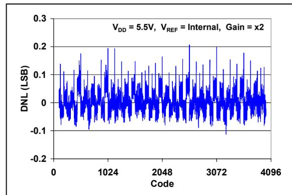
**FIGURE 2-5:** DNL vs. Code ( $T_A = +25^{\circ}\text{C}$ ).
