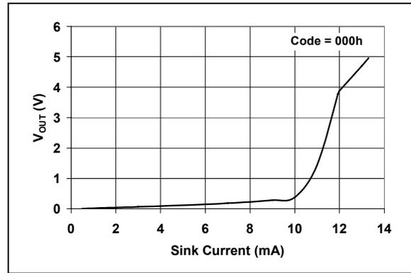
**FIGURE 2-52:** Sink Current Capability ( $V_{REF} = V_{DD}$ , Code = 000h).
