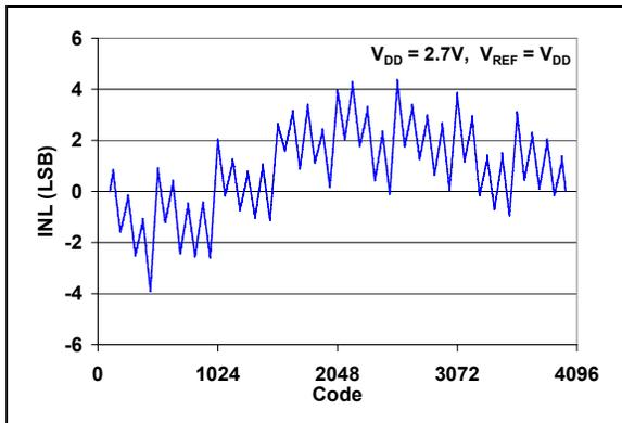
FIGURE 2-8: INL vs. Code ( $T_A = +25^\circ\text{C}$ ).
