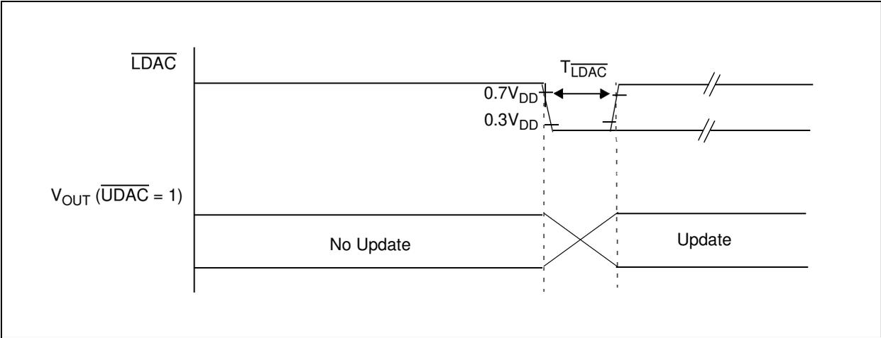
FIGURE 1-2: LDAC Pin Timing vs.  $V_{OUT}$  Update.
