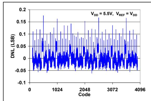
**FIGURE 2-6:** DNL vs. Code ( $T_A = +25^{\circ}\text{C}$ ).
