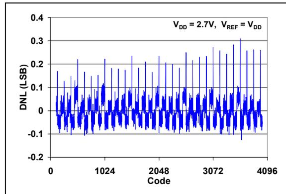
FIGURE 2-11: DNL vs. Code ( $T_A = +25^\circ\text{C}$ ).
