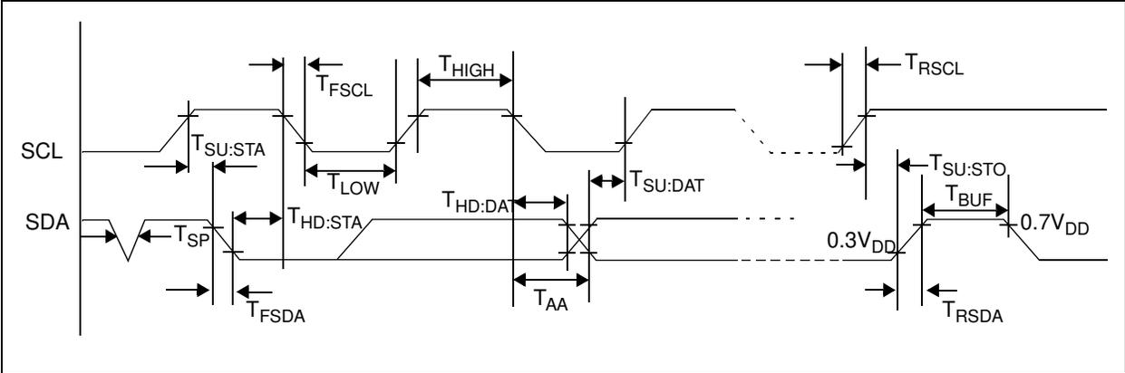
FIGURE 1-1: I<sup>2</sup>C Bus Timing Data.
