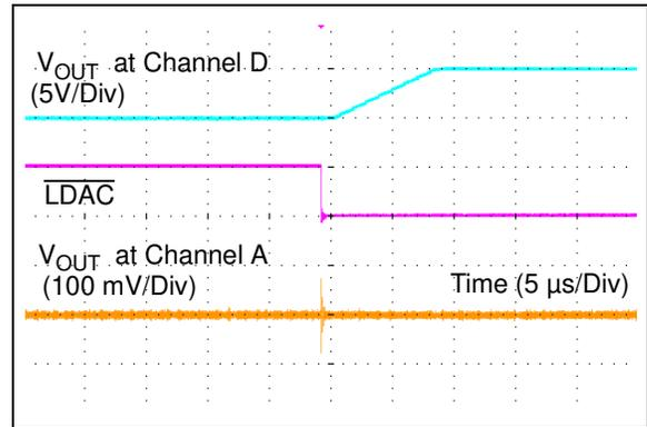
**FIGURE 2-40:** Channel Cross Talk ( $V_{REF} = V_{DD}$ ,  $V_{DD} = 5\text{V}$ ).
