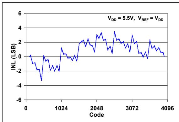
**FIGURE 2-3:** INL vs. Code ( $T_A = +25^{\circ}\text{C}$ ).
