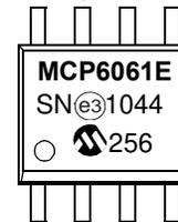
8-Lead 2x3 TDFN (MCP6061, MCP6062)
