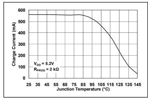
**FIGURE 5-1:** Charge Current  $(I_{OUT})$  vs. Junction Temperature  $(T_1)$ .
