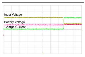
FIGURE 2-14: Overvoltage Protection Stop (50 ms/Div).
