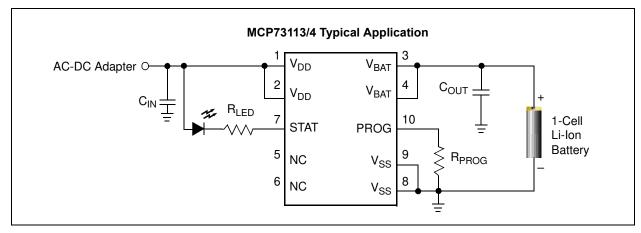
FIGURE 6-1: Typical Application Circuit.
