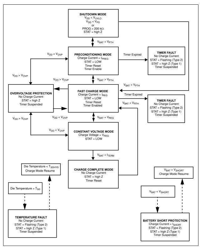
FIGURE 4-1: The MCP73113/4 Flowchart.
