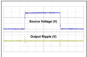
**FIGURE 2-18:** Line Transient Response  $(I_{LOAD} = 100 \text{ mA}, Output: 1.0V/Div, Source: <math>2.0V/Div)$ .
