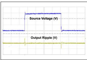
**FIGURE 2-17:** Line Transient Response  $(I_{LOAD} = 10 \text{ mA}, Output: 1.0V/Div, Source: <math>2.0V/Div)$ .
