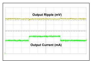
**FIGURE 2-15:** Load Transient Response  $(I_{LOAD} = 50 \text{ mA}, \text{ Output: } 100 \text{ mV/Div}, \text{ Time: } 100 \text{ µs/Div}).$
