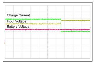
FIGURE 2-13: Overvoltage Protection Start (50 ms/Div).
