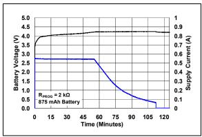
FIGURE 2-16: Complete Charge Cycle (875 mAh Li-Ion Battery.
