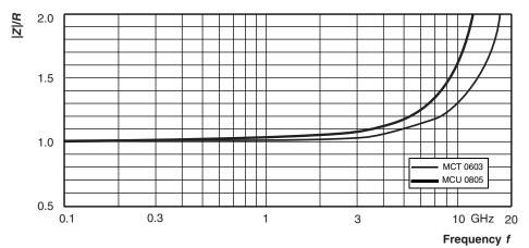
Relative impedance for 49.9  $\Omega$  chip resistor
