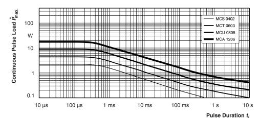
Maximum pulse load, continuous pulses; applicable if  $\bar{P} \leq P\left(\vartheta_{\text{amb}}\right)$  and  $\hat{U} \leq \hat{U}_{\text{max}}$ ; for permissible resistance change equivalent to 8000 h operation in standard operation mode
