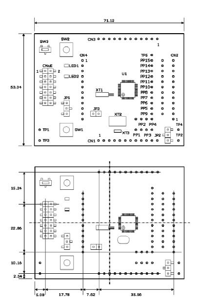
Figure 1 The ML620Q504 reference board size and external components
