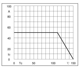
Fig5.Forward Current Derating Curve
