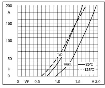
**Fig1. Forward Characteristics**
