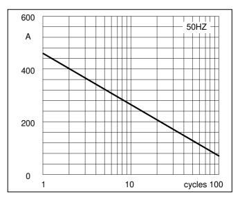
Fig4. Max Non-Repetitive Forward Surge Current
