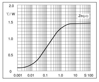
Fig3. Transient thermal impedance
