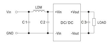
Recommended typical circuit parameters:
