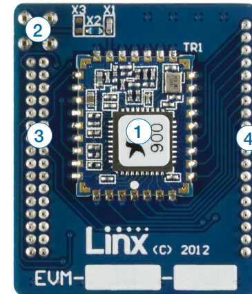
Figure 3: HumRC™ Series Transceiver Carrier Board
