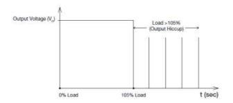
Additionally, if the  $I_{\rm O}$  is <250% but >110% for a prolong period of time (depending on the load), the Over Temperature Protection (OTP) will be activated due to high temperature on critical components. The power supply will then go into hiccup mode until the fault is removed; and, the input voltage is removed, then reapplied.
