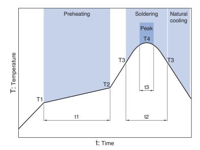
Preheating Soldering Peak Temp. Temp. Temp. Time Time Time T1 T2 t3 Т3 **T4** 150°C 180°C 60 to 120s 230°C 30 to 60s 250 to 260°C 10s max.
