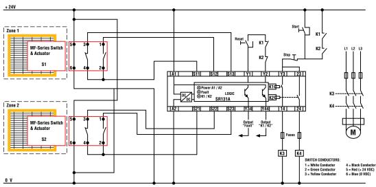
The MF Series switch and actuators are integrated with an SR131A safety monitoring relay. Each sensor has a dedicated channel for the highest level of safety.
