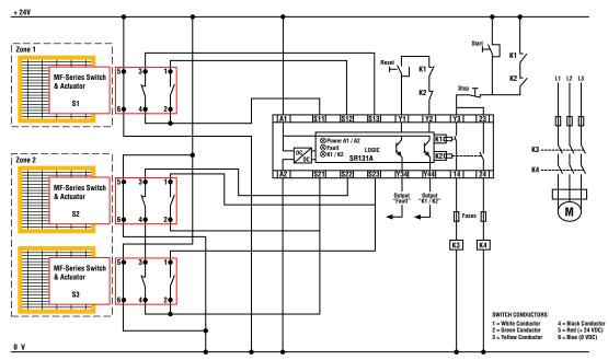
The MF Series switch and actuators are integrated with an SR131A safety monitoring relay. The safety contacts of the MF switches for zone 2 are wired in Series/Parallel. This method allows multiple gates or switches to be wired to a single channel on the safety monitoring relay or control unit.
