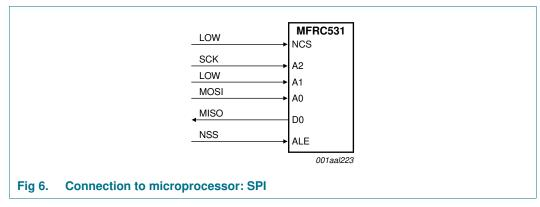
**Remark:** The SPI implementation for MFRC531 conforms to the SPI standard and ensures that the MFRC531 can only be addressed as a slave.
