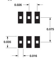
Figure 20. Recommended PCB Pad Layout for Avago's SC70 6L/SOT-363 Products.
