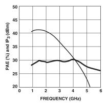
Figure 14. Power Added Efficiency and Third Order Intercept vs. Frequency ( $V_d = 3.6 \, V$ ).
