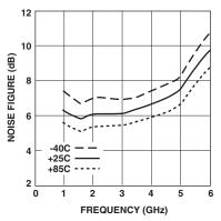
Figure 8. Noise Figure vs. Frequency and Temperature.
