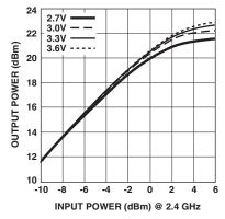
Figure 12. Output Power vs. Input Power and Voltage.
