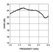
Figure 33. Small Signal Gain of the Completed 1.9 GHz Amplifier.
