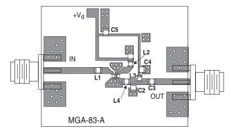
Figure 39. Completed MGA-83563 Amplifier Assembly.
