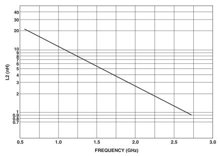
Figure 19. Values for Interstage Inductor L2.
