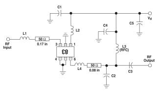
Figure 38. Schematic Diagram for the Example Amplifiers.
