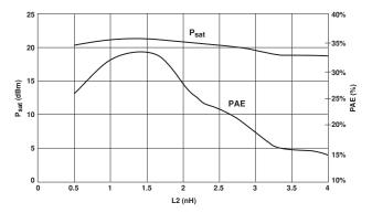
Figure 31. 2.5 GHz Psat and PAE vs. L2.
