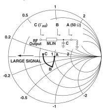
Figure 23. Initial Output Match for Small Signal.
