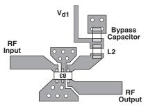
Figure 21. Basic PCB Layout.
