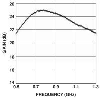
Figure 35. Small Signal Gain of the 900 MHz Amplifier.
