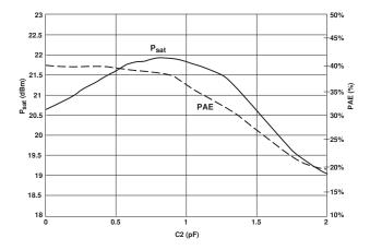
Figure 32. 2.5 GHz  $P_{\mbox{\scriptsize Sat}}$  and PAE vs. C2.
