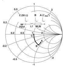
Figure 25. Initial Small Signal Input Match.
