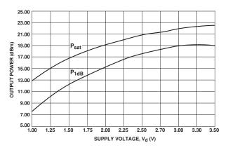
Figure 40. Output Power vs. Supply Voltage for the 2.5 GHz Amplifier.
