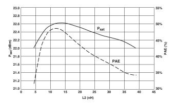
Figure 37. 900 MHz Psat and PAE vs. L2.
