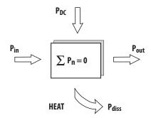
Figure 22. Thermal Representation of MGA-83563.
