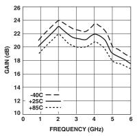
Figure 6. Gain vs. Frequency and Temperature.
