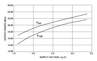
Figure 41. Output Power vs. Supply Voltage for the 900 MHz Amplifier.
