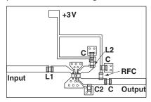
Figure 28. Completed 2.5 GHz Amplifier Assembly.
