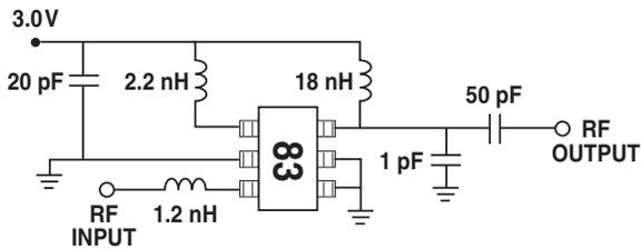
Figure 1. MGA-83563 Final Production Test Circuit.
