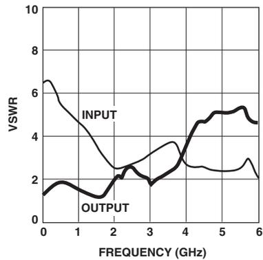
Figure 9. Input and Output VSWR vs. Frequency.
