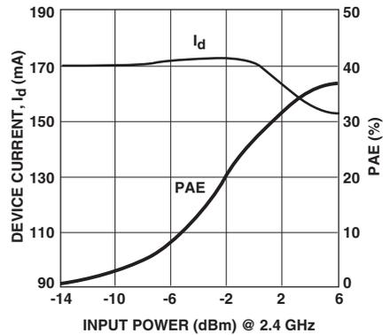
Figure 11. Device Current and Power Added Efficiency vs. Input Power.
