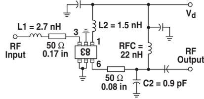
Figure 27. Schematic Diagram of 2.5 GHz Amplifier.
