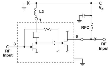
Figure 18. Interstage Inductor L2 and Bias Current.
