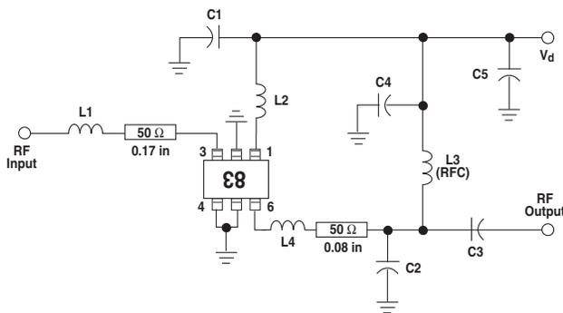
**Figure 38. Schematic Diagram for the Example Amplifiers.**
