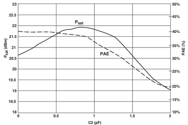
**Figure 32. 2.5 GHz  $P_{sat}$  and PAE vs. C2.**
