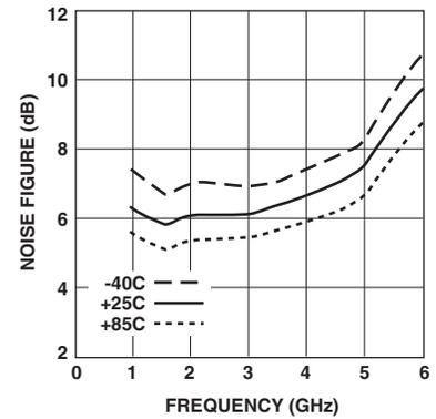
Figure 8. Noise Figure vs. Frequency and Temperature.
