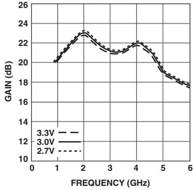
Figure 3. Tuned Gain vs. Frequency and Voltage.
