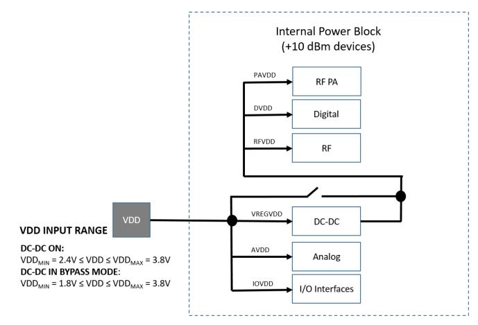
Figure 3.2. MGM12P Power Block for Modules (+10 dBm)
