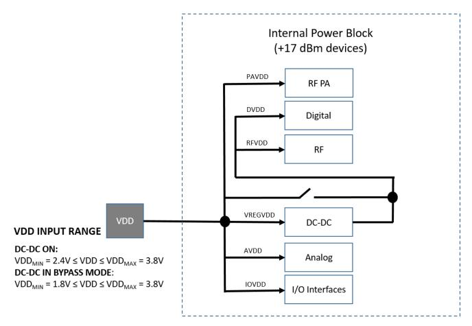
Figure 3.3. MGM12P Power Block for Modules (+17 dBm)
