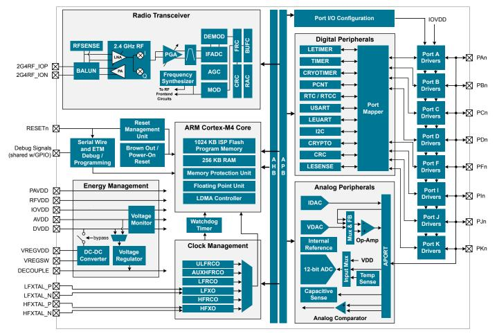
Figure 3.1. Detailed EFR32MG12 Block Diagram
