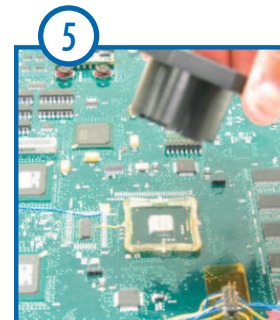
Lift to remove the Knob Tool - leaving the Frame Clip attached to the component.
