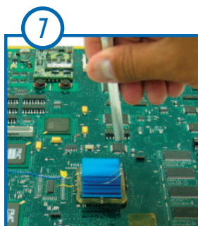
Secure the "Open End" of the Spring Clip under the lip of the frame clip.
