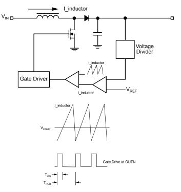
Figure 3. PWM Control Loop
