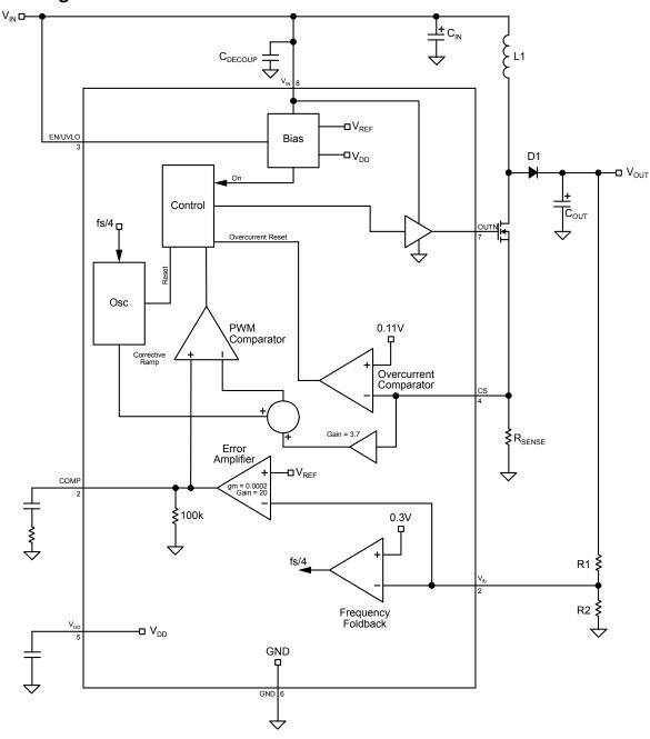
Figure 1. MIC2196 Block Diagram
