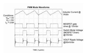
Figure 2. PWM Mode Waveforms
