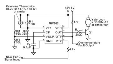
Figure 8. Typical 12V V<sub>DD</sub> Application Circuit
