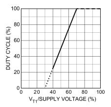
Figure 6. Control Voltage vs. Fan Speed
