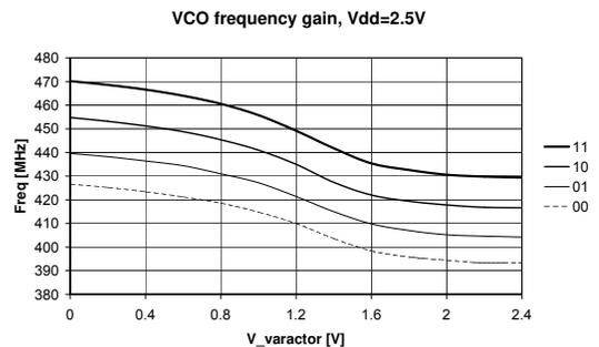
**Figure 7. RF Frequency vs. Varactor Voltage and VCO Frequency bit (V<sub>DD</sub> = 2.25V)**
