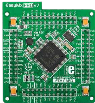
Standard 100-pin HP ETH MCU card with STM32F207VGT6
