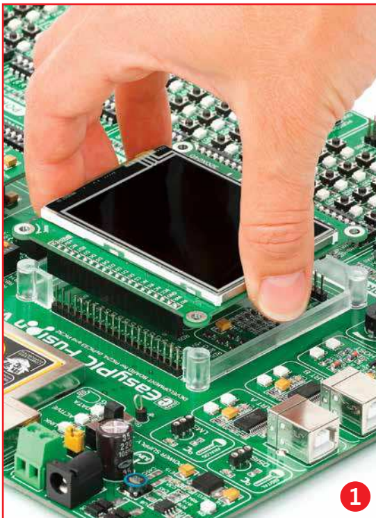
Figure 1-1: On-board GLCD socket has plastic distancer and male headers which will help you to correctly orient the MCU card before inserting.
