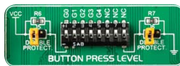
Figure 6-5: Button press level DIP switch (tri-state)
