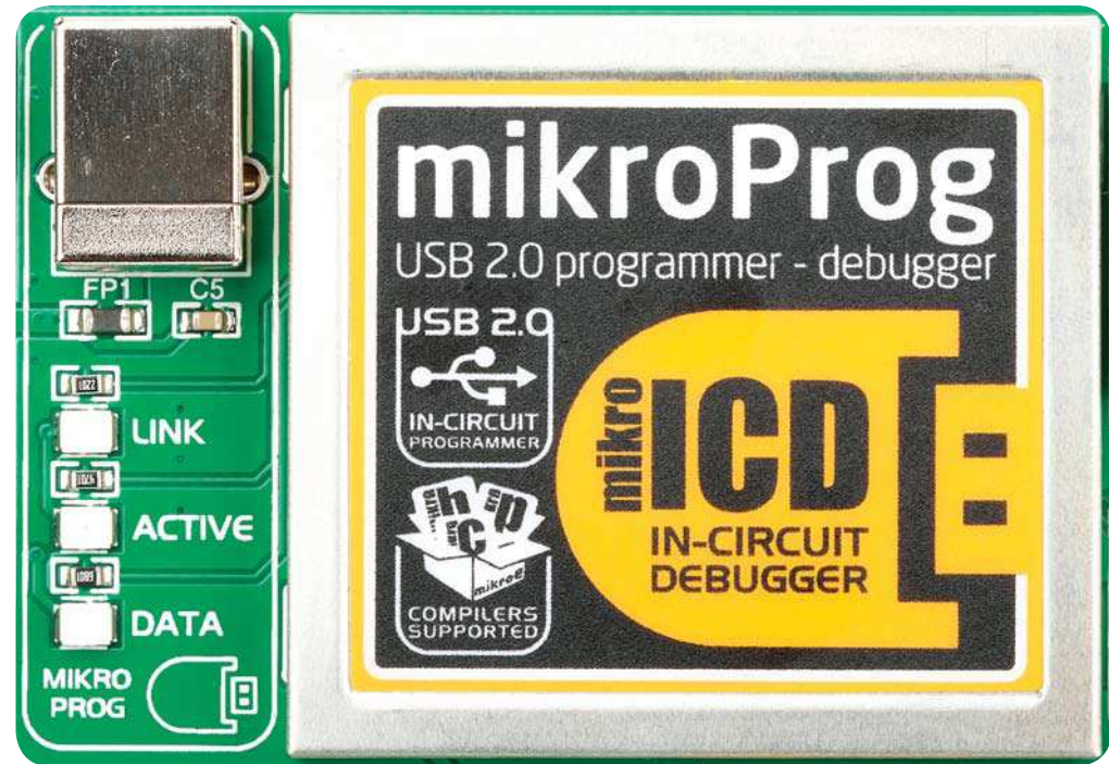
Figure 5-1: mikroProg™ is well protected under metal casing
