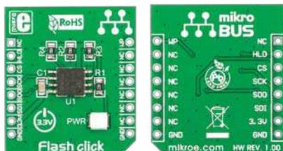
Flash Click™ is an accessory board in **mikroBUS™** form factor. It's a compact and easy solution for adding more flash memory to your device. It features **M25P80** - 8Mb serial Flash memory module with advanced hardware write protection mechanisms. Flash Click™ communicates with the target board via SPI interface. The board is designed to use 3.3V power supply only. It has a LED diode (GREEN) that indicates the presence of power supply.
