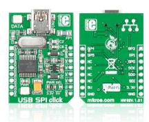
USB SPI click<sup>™</sup> is an accessory board in **mikroBUS**<sup>™</sup> form factor. It's a compact and easy solution for adding SPI serial communication via USB cable. It features **MCP2210** USB-to-SPI protocol converter with GPIO as well as USB MINI B connector. USB SPI click<sup>™</sup> communicates with target board via SPI interface as a master device. The board is designed to use 3.3V or 5V power supply. It has a LED diode (GREEN) that indicates the presence of power supply.
