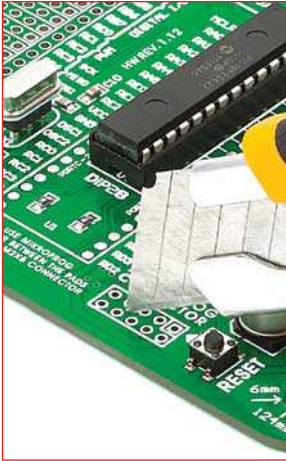
Figure 3-2: cutting copper between pads between pads
