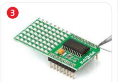
Turn the board upward again. Make sure to align the headers so that they are perpendicular to the board, then solder the pins carefully.
