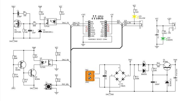
Target board microcontroller can receive a signal from DALI peripherals via interrupt pin
