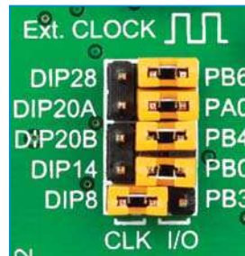
Figure 4-10: Position of the jumpers for DIP8
