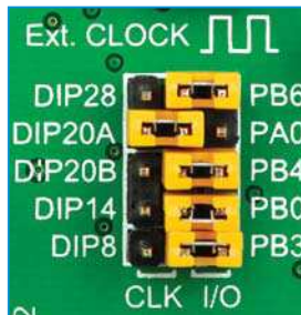
Figure 4-7: Position of the jumpers for DIP20A
