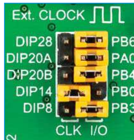
Figure 4-9: Position of the jumpers for DIP14
