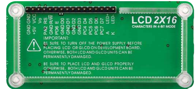
Figure 10-1: On-board LCD 2x16 display connector
