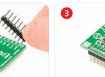
Turn the board upside down so that bottom side is facing you upwards. Place shorter parts of the header pins in both soldering pad locations. Turn the board upward again. Make sure to align the headers so that they are perpendicular to the board, then solder the pins carefully.
