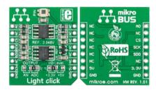
Light Click" is an accessory board in mikroBUS" form factor. It's a compact and easy solution for adding light sensor to your design. It features PD15-22C-TR8 PIN photodiode, MAX6106 voltage reference and MCP3201 ADC with SPI interface. Light Click" communicates with the target board microcontroller via mikroBUS" SPI (MISO, SCK, CS) and AN lines. The board is designed to use 3.3V and 5V power supply. LED diode (GREEN) indicates the presence of power supply.
