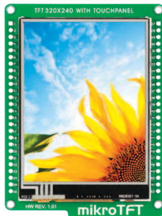
Figure 2: mikroTFT display board
