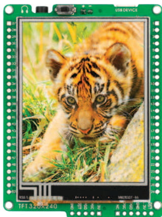
Figure 1: mikromedia for PIC32 development board
