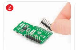
Turn the board upside down so that bottom side is facing you upwards. Place shorter pins of the header into the appropriate soldering pads.
