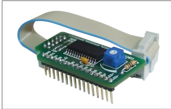
Figure 1: Serial LCD Adapter additional board
