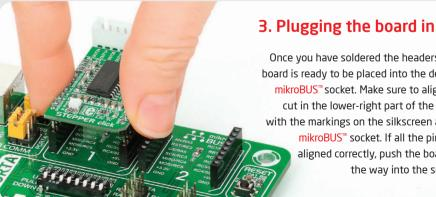
Once you have soldered the headers your board is ready to be placed into the desired mikroBUS<sup>™</sup> socket. Make sure to align the cut in the lower-right part of the board with the markings on the silkscreen at the mikroBUS™ socket. If all the pins are aligned correctly, push the board all
