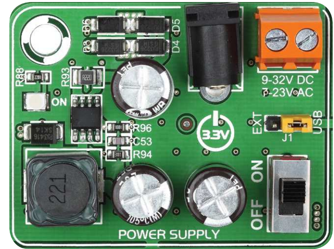
Figure 3-1: Power supply unit of EasyMx PRO™ v7 for Tiva™ C Series
