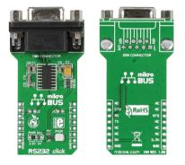
RS232 click<sup>™</sup> is a simple solution for adding RS232 serial communications to your design. The board features a standard RS232 DB9 port and a MAX3232 IC, along with a **mikroBUS<sup>™</sup>** host socket, three jumpers and a power indicator LED. RS232 click<sup>™</sup> communicates with the target board through mikroBUS<sup>™</sup> RX (RXD), TX (TXD), CS (RTS), and INT (CTS) lines. RS232 click<sup>™</sup> is designed to use either a 3.3V or 5V power supply.
