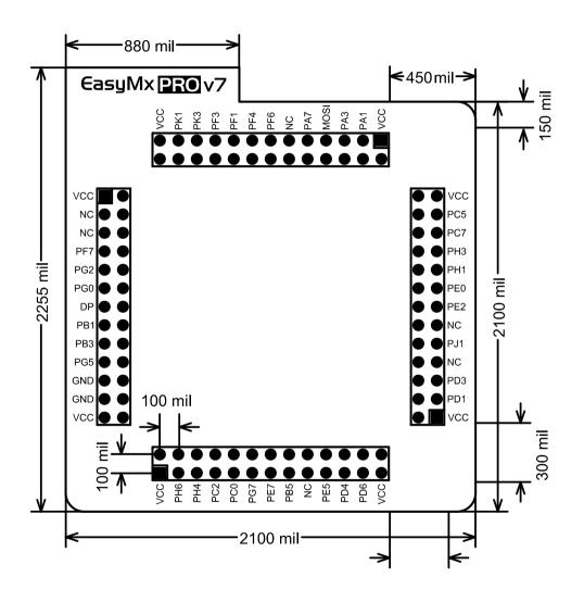
Figure 3: MCU card dimensions. Values are in mils.
