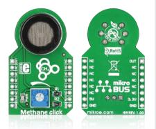
Methane click<sup>™</sup> is a simple solution for adding a high sensitivity methane  $(CH_4)$ sensor to your design. It's suitable for designing gas leakage equipment. The board features an MQ-4 sensor, a calibration potentiometer, a mikroBUS<sup>™</sup> host socket, two jumpers and a power indicator LED. Methane click<sup>™</sup> communicates with the target board through mikroBUS<sup>™</sup> AN (OUT) line. Methane click<sup>™</sup> is designed to use a 5V power supply only.
