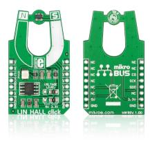
LIN HALL click<sup>™</sup> is a simple solution for adding a linear Hall sensor to your design. It carries an MLX90242 linear Hall sensor IC (with built-in active error correction circuitry) and an MCP3201 12-bit ADC. LIN HALL click<sup>™</sup> communicates with the target board through the **mikroBUS**<sup>™</sup> SPI lines (CS, SCK, MISO). The board is designed to use either a 3.3V or 5V power supply.
