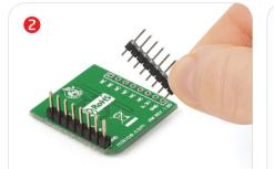
Turn the board upside down so that the bottom side is facing you upwards. Place shorter pins of the header into the appropriate soldering pads.
