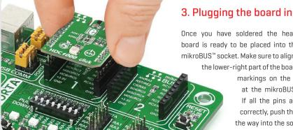
Once you have soldered the headers your board is ready to be placed into the desired
