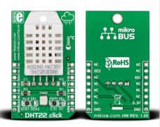
DHT22 click\*\* is a temperature and humidity measurement board carrying the AM2302 sensor (also known as DHT22). It's a low cost reliable sensor that communicates with the target board microcontroller through a single Serial Data Line. You can choose between the mikroBUS\*\* CS or INT pins for communicating with the target board microcontroller. The board is designed to use either a 3.3V or a 5V power supply.
